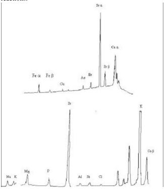
Figure 3. Identification of the main elements presents in the structure of *Sargassum* sp. biomass by X-ray fluorescence.
